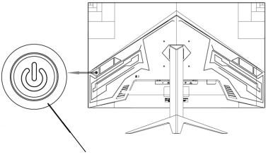
Power Switch (To Power-Off the Display please hold Button for 3 seconds)
